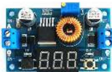
DC-DC converter step down in 3V – 40V Out 5V – 36V 4A
