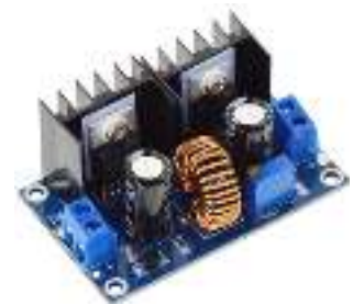
DC-DC converter step down in 3V – 40V Out 5V – 36V 8A
